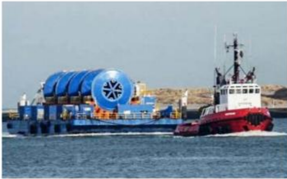
Figure-3 Cable Laying Vessel
