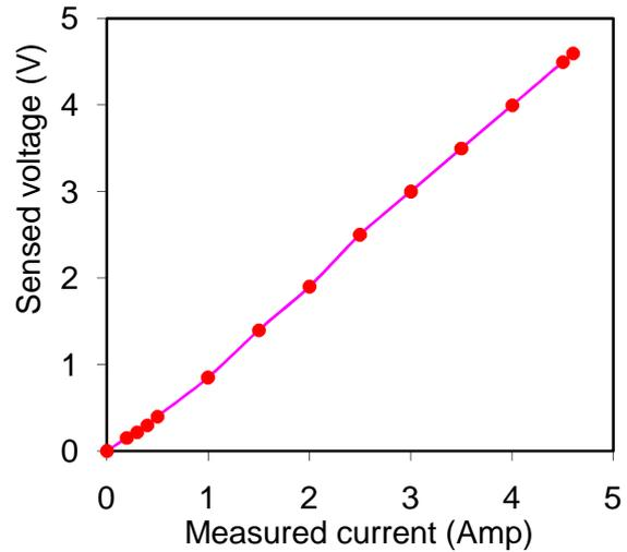
Fig. 6(a) Plot of sensed voltage versus measured current
