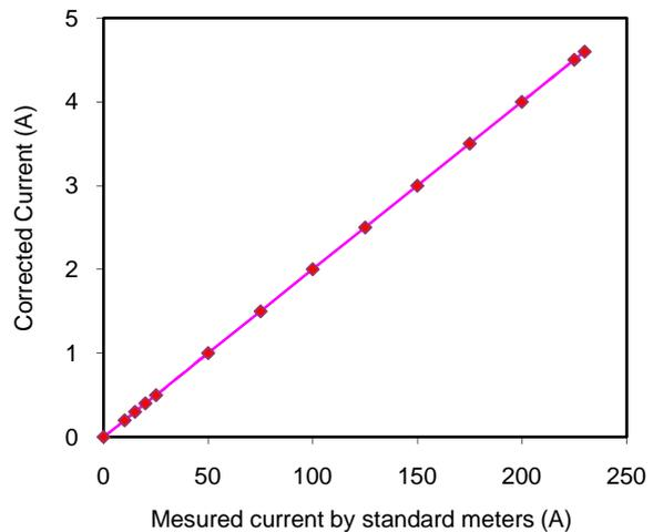
Fig. 6(b) Plot of corrected current versus measured current by standard meters.
