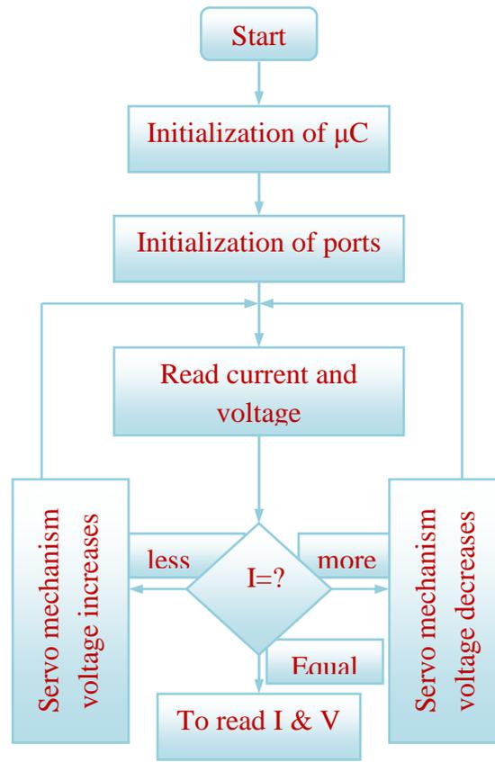
Fig. 4 Flow chart the system software
