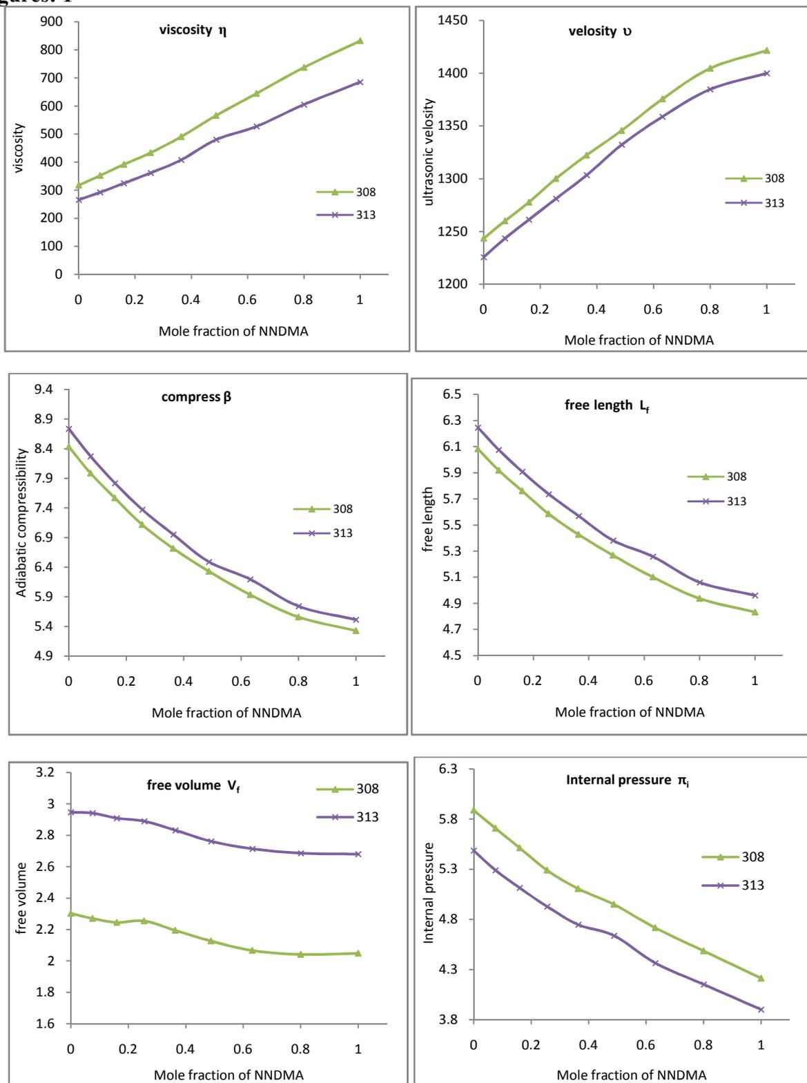
**Figure 01:-** Plots of ultrasonic velocity, viscosity, adiabatic compressibility ( $\beta_a$ ), free length ( $L_f$ ), free volume ( $V_f$ ) and internal pressure ( $\pi_i$ ) and their excess values, for N,N-dimethylacetamide + Acetonitrile mixture at 308.15K and 313.15K temperature.
