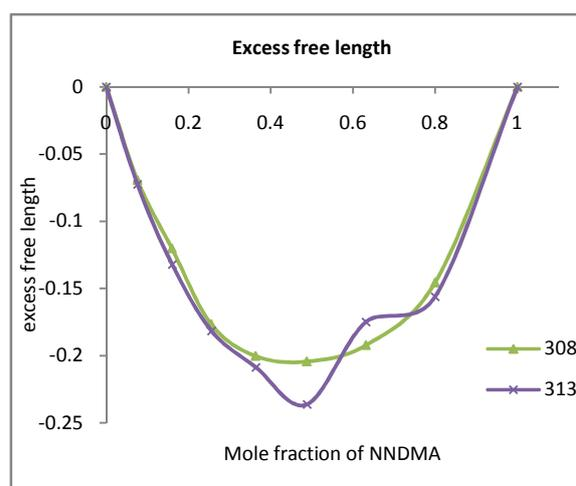
2: Plot of excess free length versus Mole fraction of NNDMA
