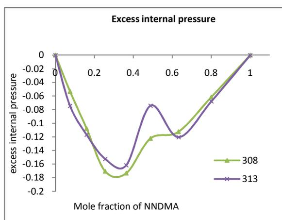
3: Plot of excess internal pressure versus mole fraction of NNDMA
