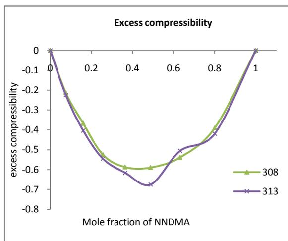
1: Plot of excess adiabatic Compressibility versus Mole fraction of NNDMA
