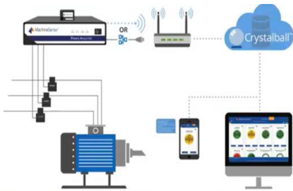
Fig.7 Working of Power network analyser.
